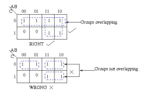
7. Groups may wrap around the table. The leftmost cell in a row may be grouped with the rightmost cell and the top cell in a column may be grouped with the bottom cell.
